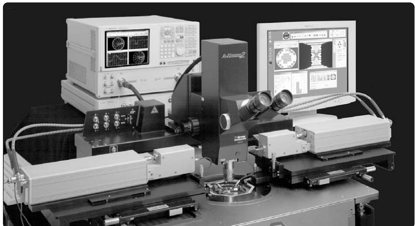
Figure 2. N5250A 110 GHz mm-wave system with Cascade Microtech's probe station.
